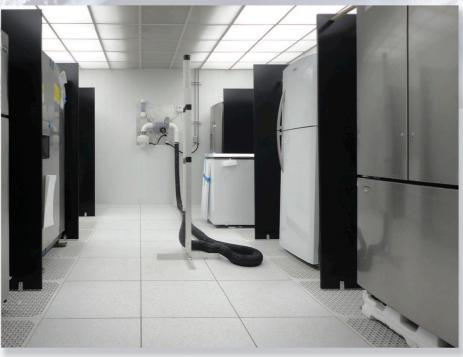
The chamber shall be equipped with a raised floor that provides an adequately sized floor cavity to accommodate the circulating conditioned air. The floor shall allow for against-the wall air plenums that will take the circulating conditioned air from the floor cavity to the ceiling.
