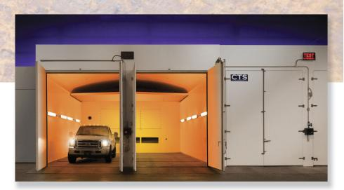
The Corrosion Salt Spray Vehicle Chamber designed to provide accelerated corrosion life testing of body, frame, undercarriage components of passenger cars and trucks. The facility is capable of quickly cycling from hot, humid to hot, dry conditions to cooler dry conditions and back again. Salt solutions are injected in front, above and under the vehicle to simulate on-road salt conditions.
