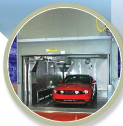
The Evaporative Emissions Test System, Variable Volume/Variable Temperature (VV/VTS) Sealed Housing for Evaporative Determination (SHED), is designed for use in measuring automotive diurnal evaporative hydrocarbon (HC) emissions from non-operating test vehicles.
